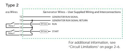
Figure 2-8 Type 2 Connection Diagram
