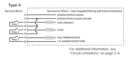
Figure 2-10 Type 4 Connection Diagram
