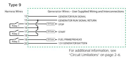
Figure 2-17 Type 9 Connection Diagram
