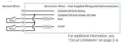
Figure 2-16 Type 8 Connection Diagram (three-wire)
