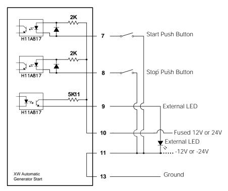
Figure 2-23 External ON/OFF Switch and LED Wiring Diagram
