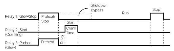
Figure C-9 GlowStop Mode Timing Diagram
