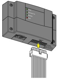
Figure 2-24 AGS External Connections
