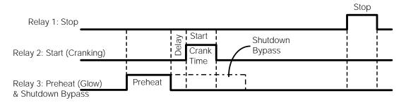
Figure C-10 StartStop Mode Timing Diagram
