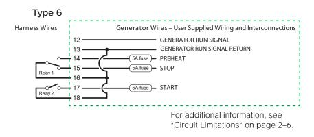
Figure 2-12 Type 6 Connection Diagram
