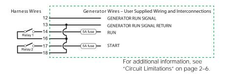
Figure 2-14 Type 7 Connection Diagram (three-wire)
