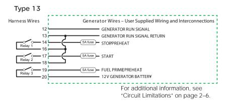
Figure 2-21 Type 13 Connection Diagram
