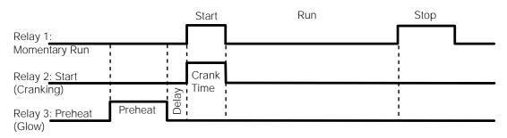
Figure C-8 MomentaryRun Mode Timing Diagram
