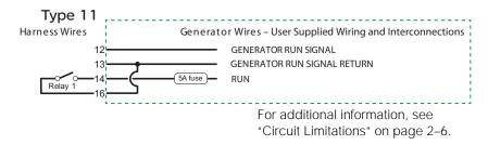
Figure 2-19 Type 11 Connection Diagram
