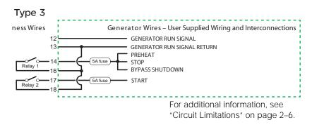
Figure 2-9 Type 3 Connection Diagram
