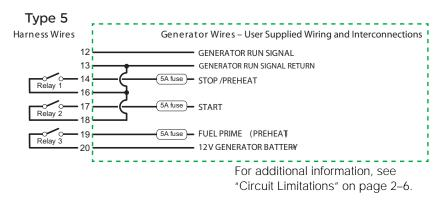
Figure 2-11 Type 5 Connection Diagram
