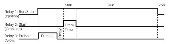
Figure C-7 RunMode Timing Diagram
