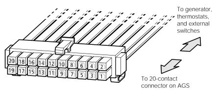
Figure 2-6 AGS Wiring Harness
