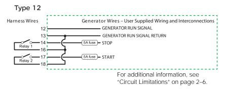
Figure 2-20 Type 12 Connection Diagram
