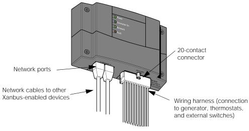
Figure 2-5 AGS External Connections
