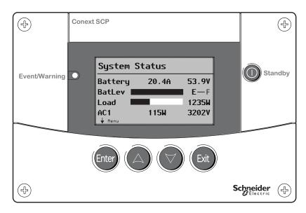
Figure 3-28 SCP System Status Screen and Navigation Buttons
