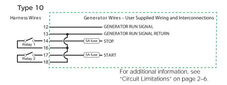
Figure 2-18 Type 10 Connection Diagram
