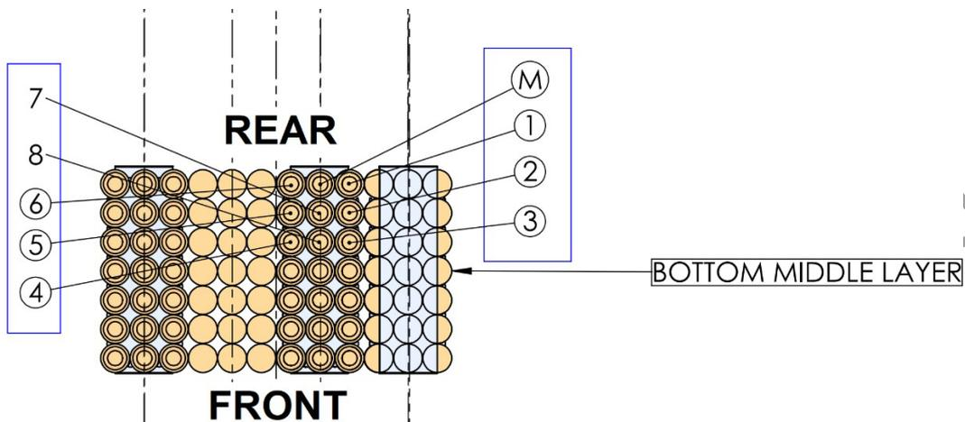
Figure 4 – Cell No. Identification for this report (top view).
