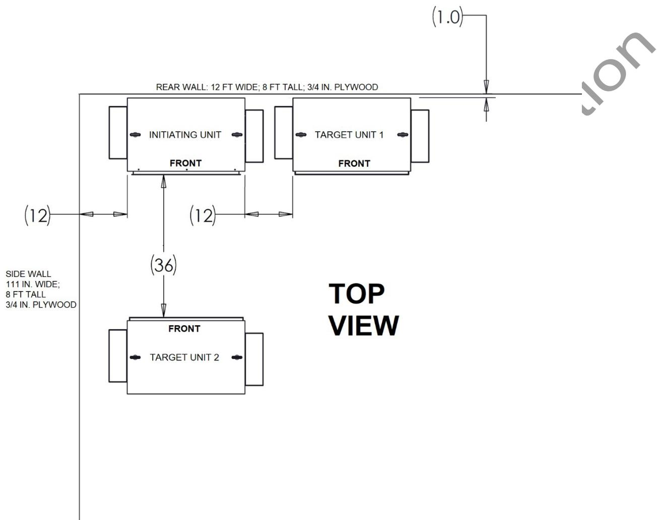
Figure 1 – Orientation of Initiating and Target Units (12 in. soffit not shown; located at top end of side and rear wall)
