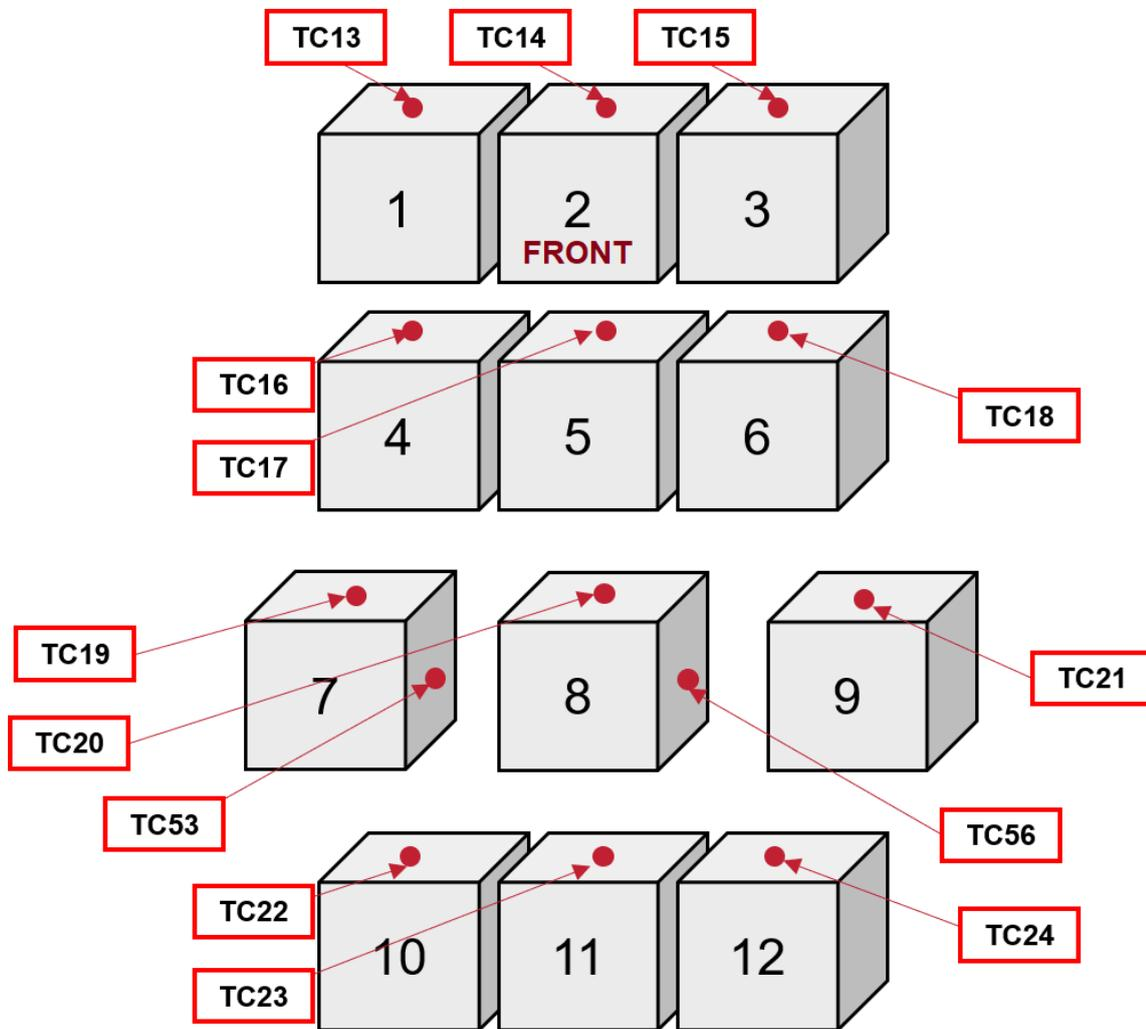
Figure 1 – Thermocouple Locations on top of Modules inside Initiating Unit (TC 54 and 55 not shown above due to viewing angle)
