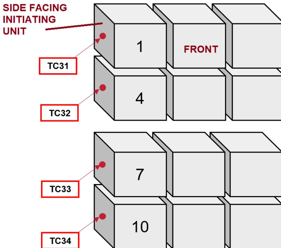
Figure 1 – Thermocouple Locations on Modules inside Target Unit 1
