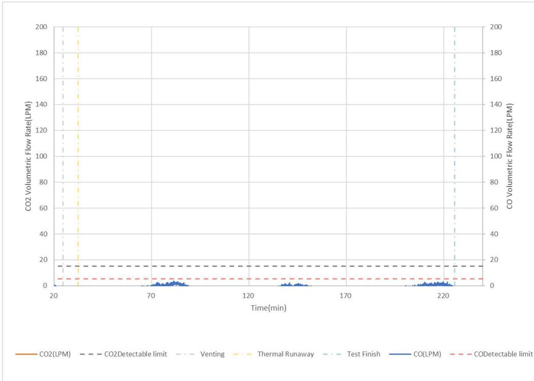
Figure 1 – Volumetric Flowrates of gasses (CO<sub>2</sub> and CO)
