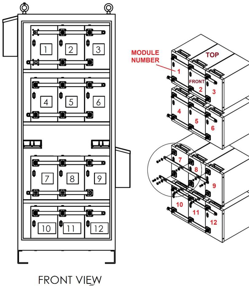
Figure 1 – Internal Layout of Unit
