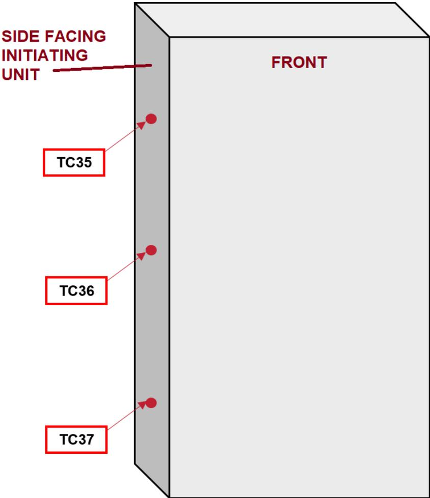
Figure 2 – Thermocouple Locations External Surface of Target Unit 1
