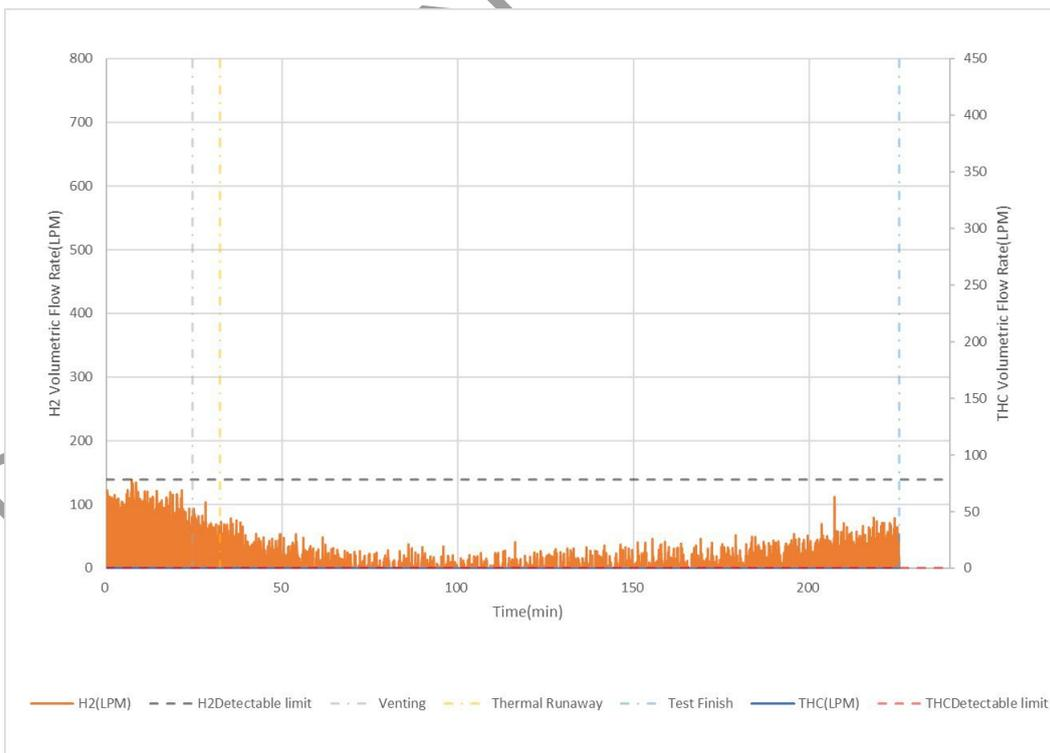
Figure 2 – Volumetric Flowrates of gasses (THC and H<sub>2</sub>)
