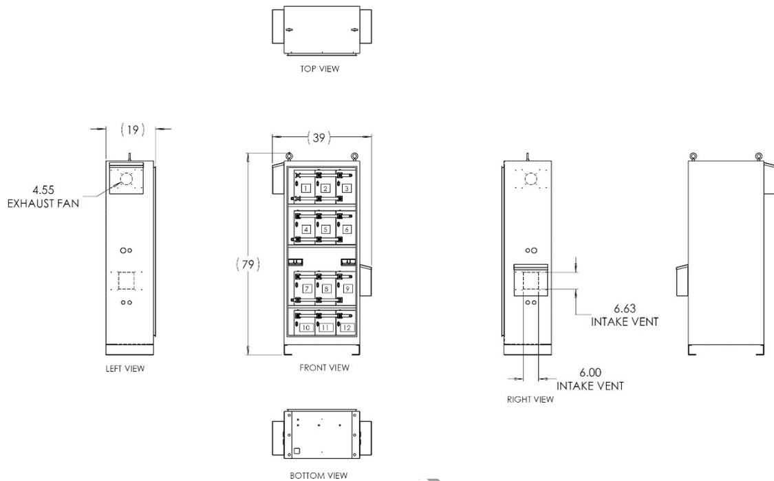
Figure 3 – Detailed Drawing of Cabinet
