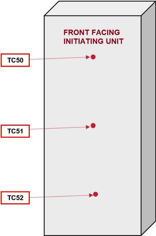
Figure 2 – Thermocouple Locations External Surface of Target Unit 2
