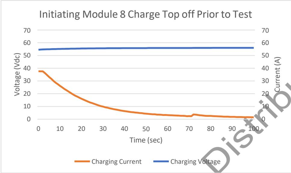
Figure 9 – Initiating Module 8 Charge Top off Prior to Test
