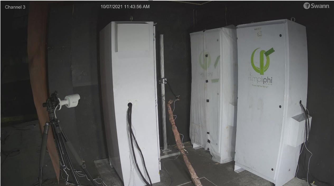
Figure 8 – Thermal Runaway of Cell No. 2 (00:34:14)
