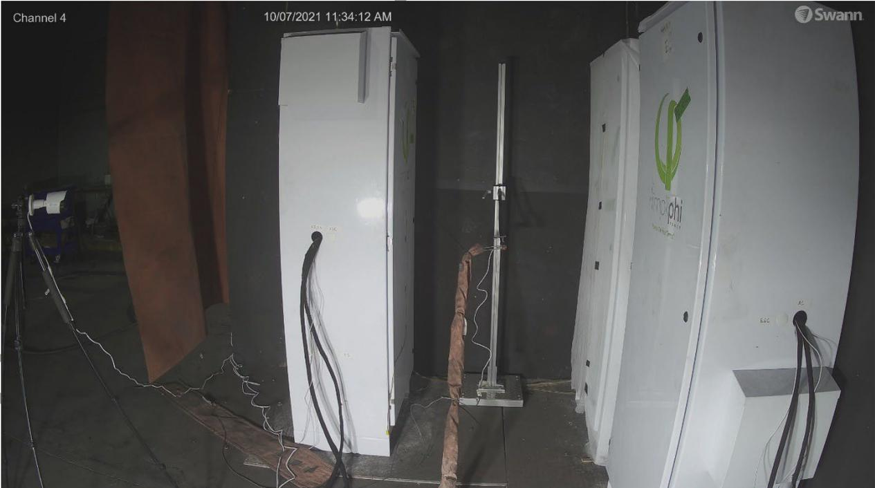
Figure 2 – Venting of Cell No. 6 (00:24:30)
