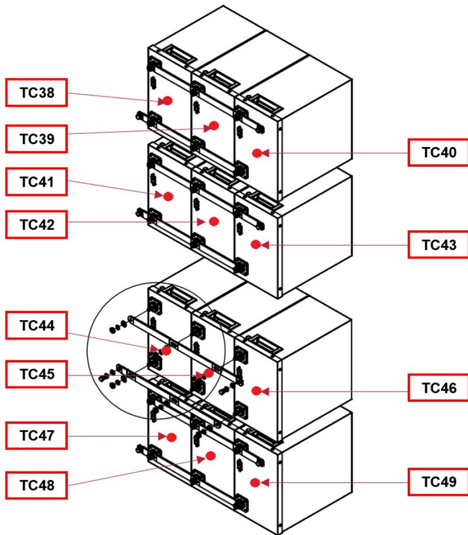
Figure 1 – Thermocouple Locations on Modules inside Target Unit 2
