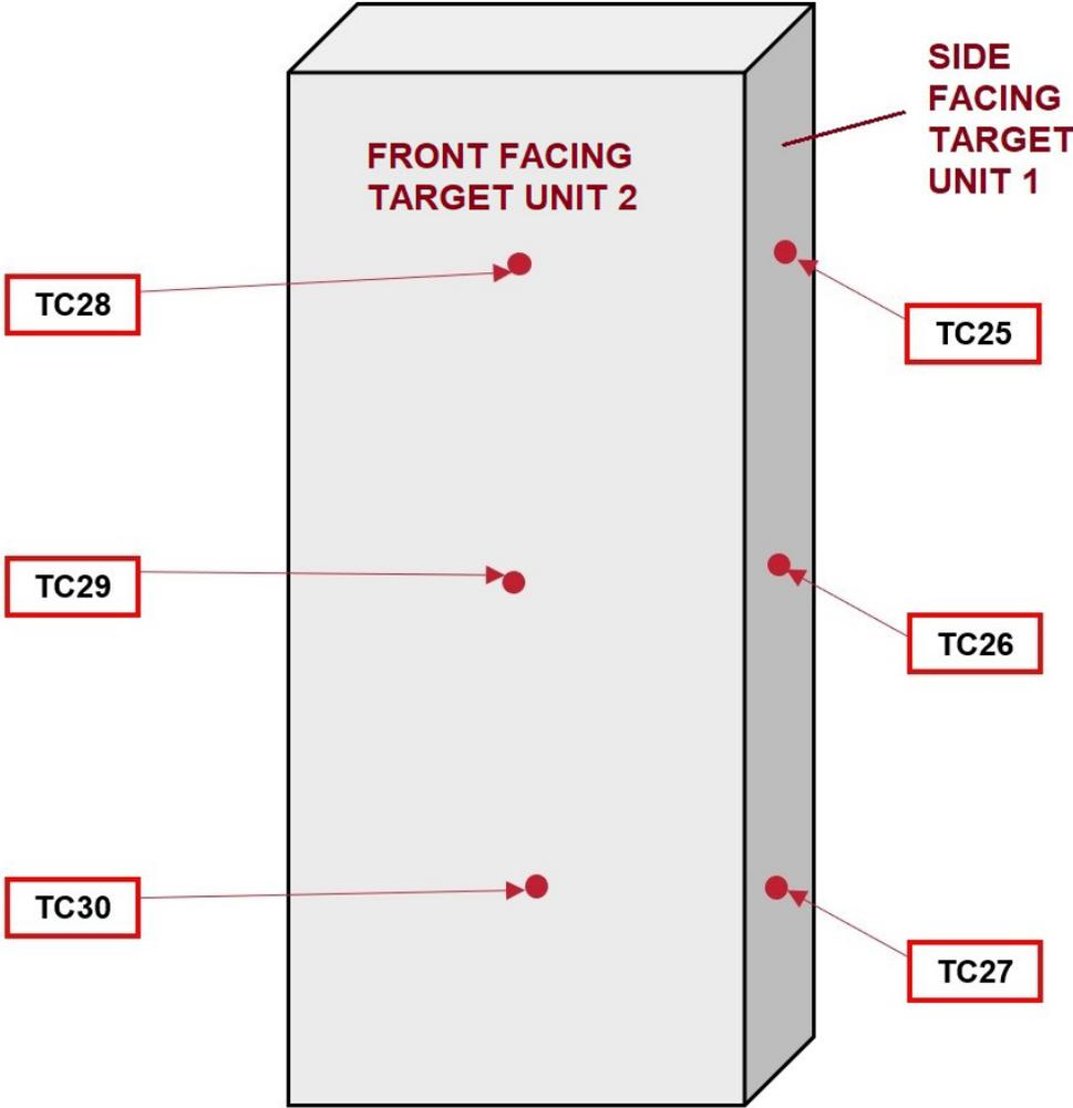
Figure 2 – Thermocouple Locations External Surface of Initiating Unit
